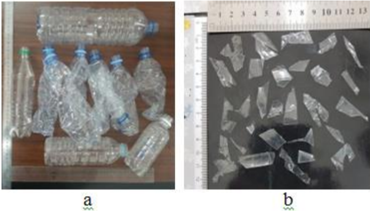
Fig 2: (a) The waste PET and (b) shredded PET waste
